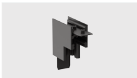
L-shaped(Inward) Model:MT11-L90N-MH11 Material:AL6063-T5 Size: L39.5xW39.5xH19mm Applicable model:TLS-MT11-HX0
