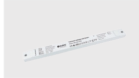
Power supply Model:BN-V48-150P Size:L350xW30xH18mm Input voltage:220-240VAC Output:DC48V Power:150W Applicable model:All track
